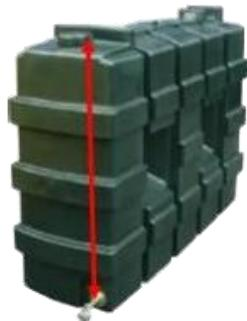
**Note:** The bottom of the pipe should be a minimum of 5cm from the base (floor) of the tank to prevent it from touching in the case of tank dimensional changes due to temperature etc.
