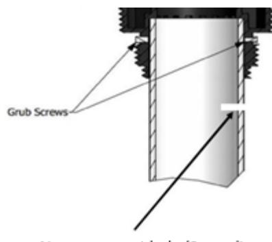
**Note:** Depending on the weight, length and surface finish of the pipe, it may be necessary to glue it into position. In this case a hole should be drilled near the top of the waveguide pipe, just below the adapter, to ensure that any trapped air can exit.
